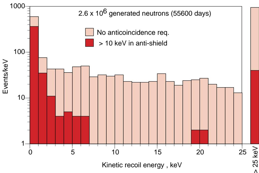
**Figure 12.** Recoil energy spectrum for a fission neutron source and  $2 \times 10^{-3}$  n/s in the walls of the cryostat, presumably due to Th and U contamination. The effect of the anti-coincidence shield, in which a an energy deposition > 10 keV has been imposed is evident.
