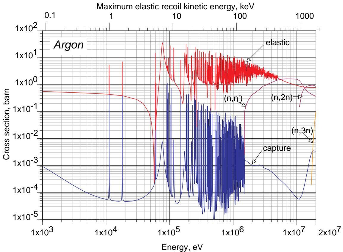
**Figure 11.** Neutron cross sections in natural Argon. The maximum energy of the elastic recoil is also shown. We note the complex cross section behaviour in the region of recoils of interest ( $10 \div 100$  keV).
