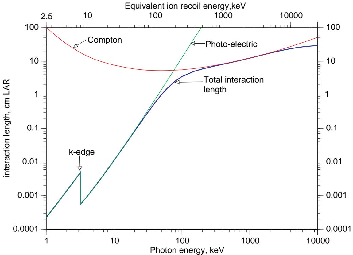
**Figure 13.** Interaction length in cm of liquid Argon as a function of the photon energy. The equivalent energy of a WIMP recoil (scintillation light) is also shown. At low energies, the photo-effect dominates, while at high energies Compton effect takes over. Above a few MeV, pair production (not shown) becomes relevant.
