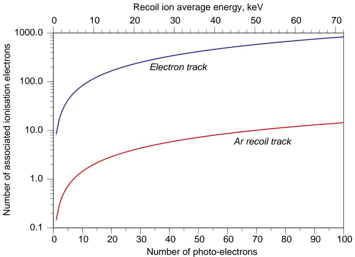
**Figure 6.** Calculated number of associated ionisation electrons as a function of the number of scintillation photo-electrons collected in Argon for recoil tracks and for (background)  $\gamma/e$  events with the same average scintillation light collected.
