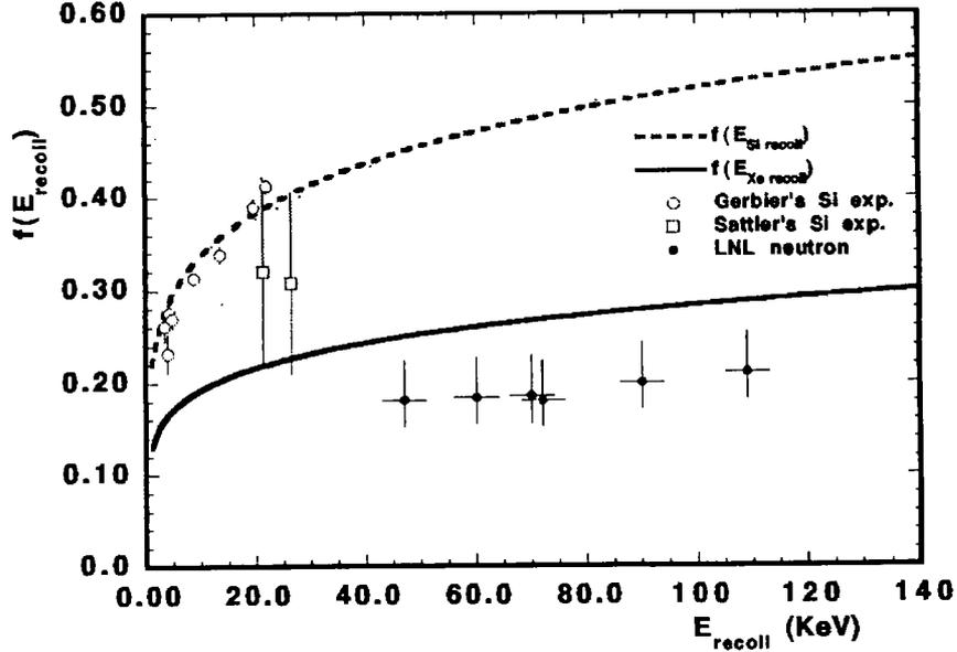
**Figure 4.** Relative scintillation efficiency in liquid Xenon as a function of the Xenon recoil energy. Full circles are ICARUS data [5], open circles and squares are data points on Silicon from ref. [6] and [7] respectively. The curve represents the theory of Lindhard et al [8] for Xenon and Silicon respectively.
