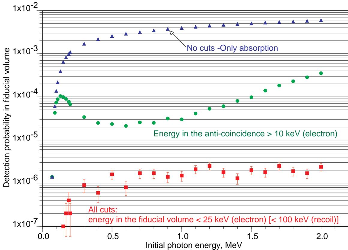
**Figure 14.** Detection probability for a single hit in the sensitive volume of a photon emitted by the cryostat walls, as a function of its energy. The effect of the cuts is displayed
