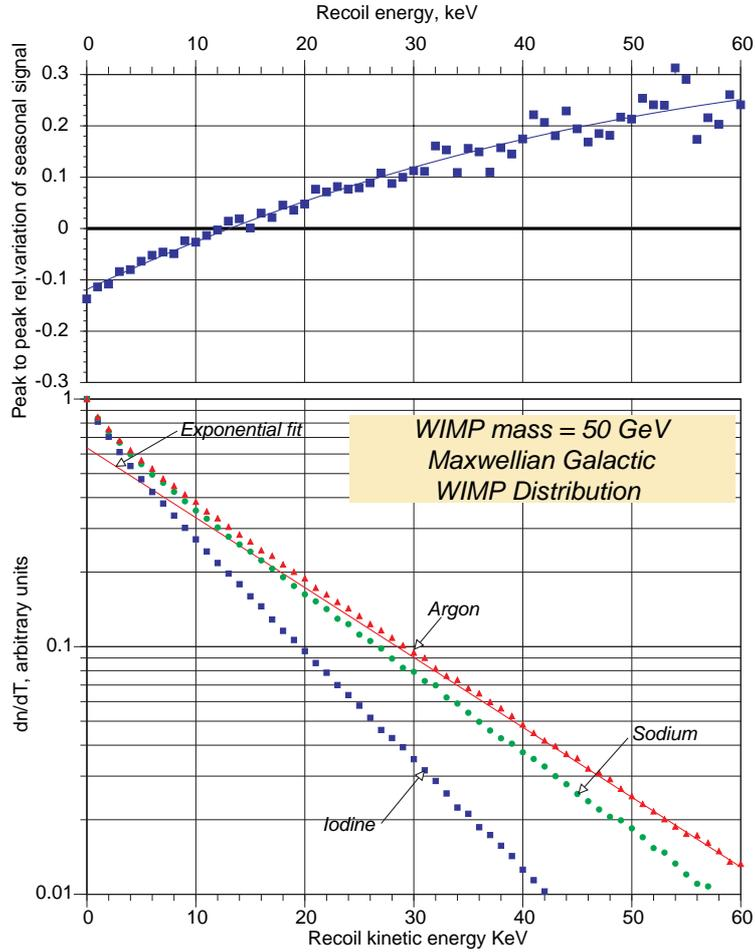
**Figure 3.** Monte Carlo prediction for WIMPS recoil spectrum in three different target elements. The WIMPS kinematical model is based on a truncated Maxwellian distribution in the galactic rest frame with a characteristic velocity of 220 km/s. For other parameters, see Table 1.
