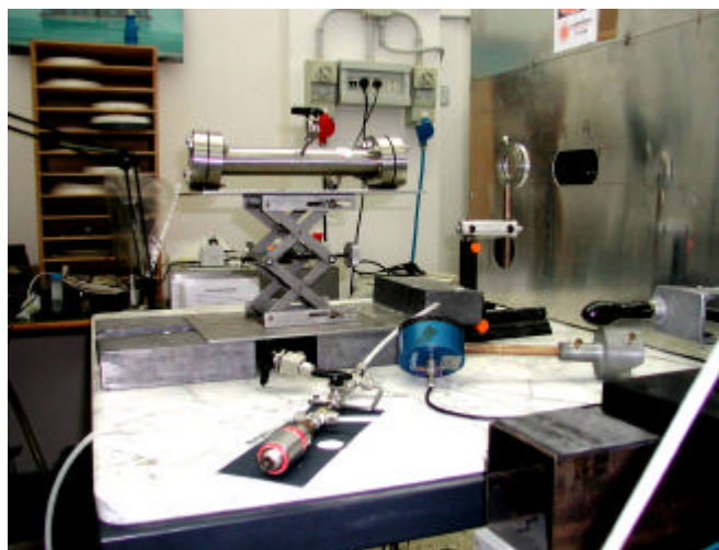
Fig.1- Experimental set-up- W: quartz window; T-Pd sample; L-lens; ND: Neutral density filters-
