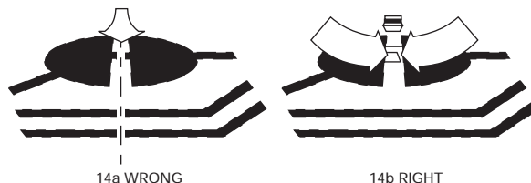
Figure 14 How to cut PCB links
